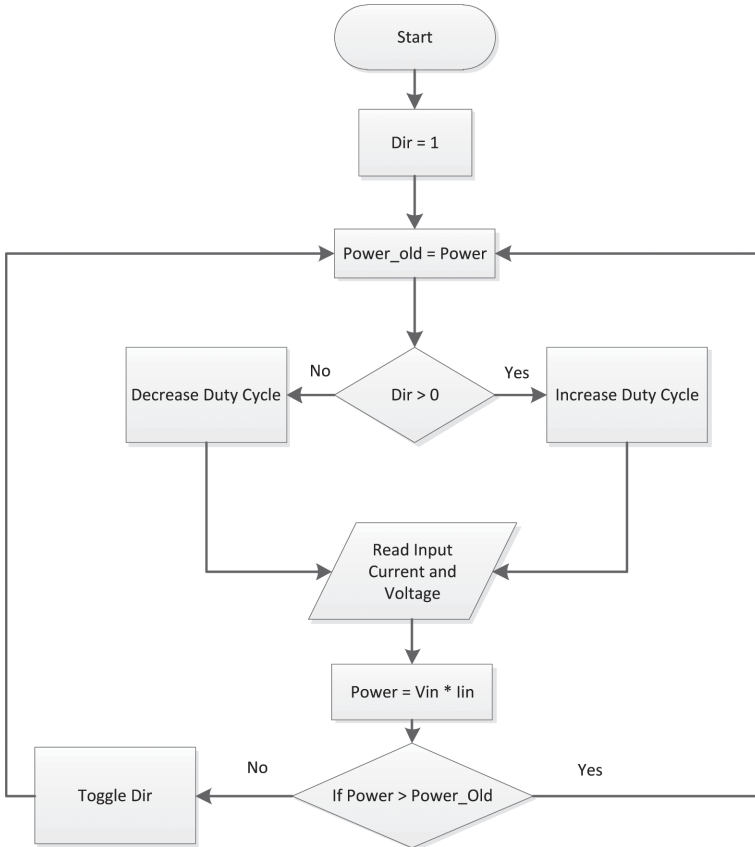
Figure 8.7 Hill climbing logic MPPT.
