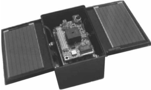
Figure 8.19 Heliomote with solar panels. 4
