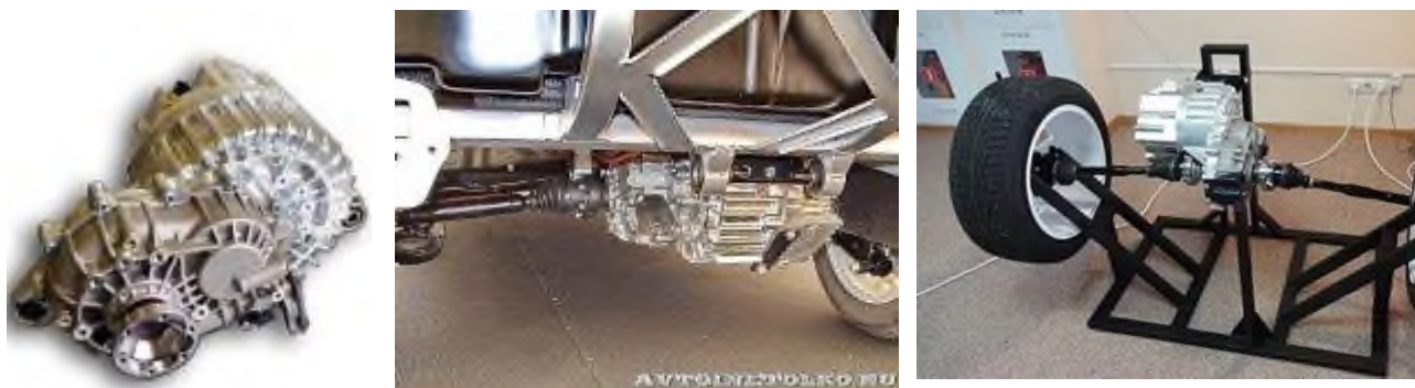
14.12-rasm. “Dvigatel-ishchi organ” tipidagi yuritmalar
