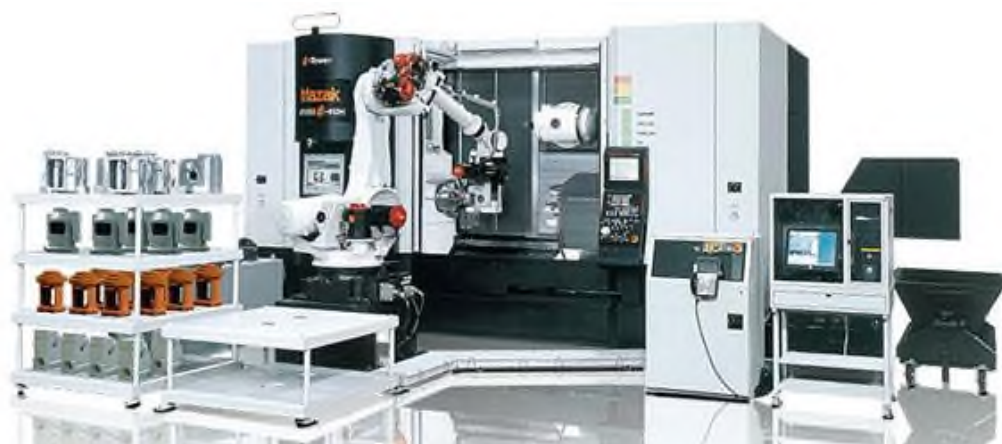
3.7-rasm. Moslashuvchan ishlab chiqarish jihozi
