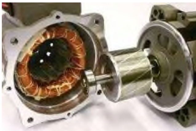
7.5-rasm. Elektrdvigatel tuzilishi
