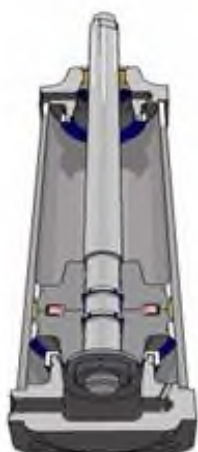
8.14-rasm. 3D-formatdagi pnevmatik porshenli silindr qirqimi
