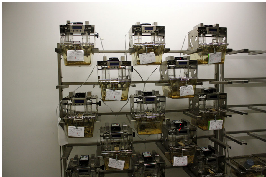
FIGURE 31.3 Overview of the drinkometer system to study alcohol drinking patterns in mice. This system is a fully automated, highly precise monitoring system for alcohol drinking in mice in the home cage that allows for detecting micro-drinking and circadian drinking patterns. The system is used to monitor simultaneously water and alcohol consumption as well as motor activity at high accuracy and in a high time resolution.
