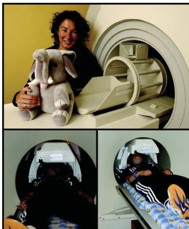
Figure 18.5 Pictures of various MR simulators. The top panel shows a scanner simulator that includes a replica of the head coil and stimulus display device just above. The bottom panels show a 10-year-old male in the scanner simulator, wearing headphones and looking at the video display where, during the simulation, a movie is playing or, during a study, the experimental stimuli are projected.
