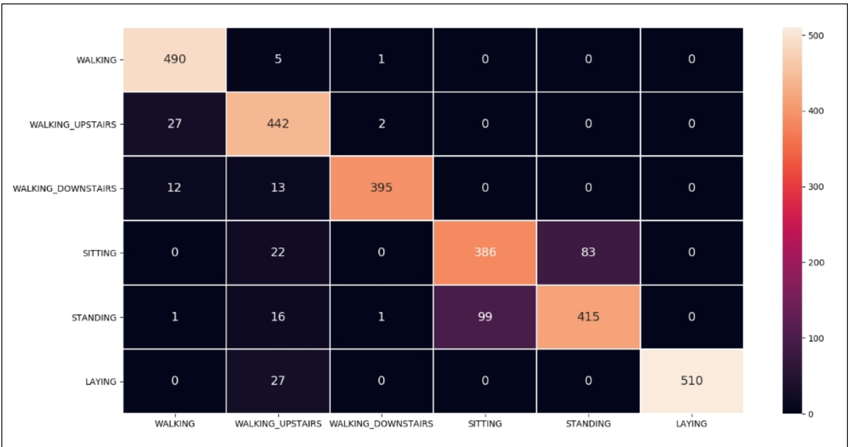
Figure 27: Multiclass confusion matrix (predicted vs actual)
