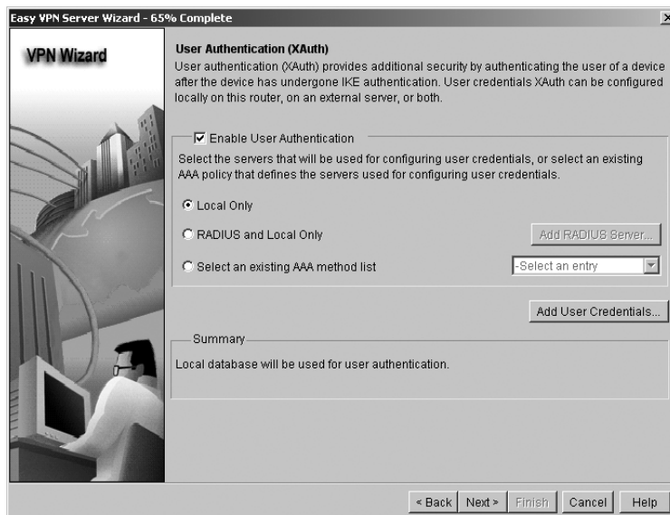
FIGURE 12.17 Cisco Router and Security Device Manager Easy VPN Server Wizard User Authentication (XAuth) screen
