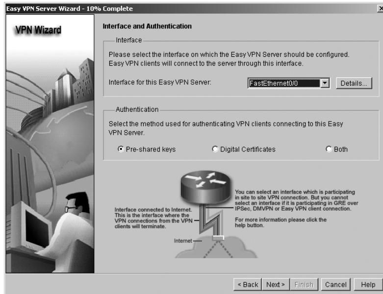
FIGURE 12.13 Cisco Router and Security Device Manager Easy VPN Server Wizard Interface And Authentication screen
