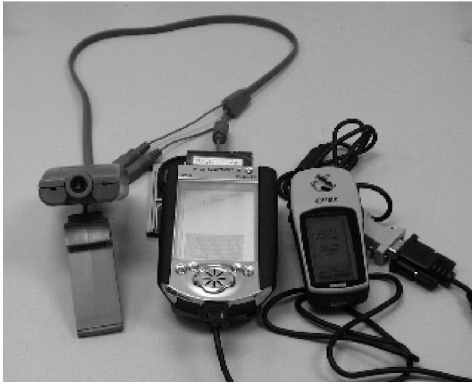
FIGURE 13.9 Prototype node with video camera and GPS receiver attached.
