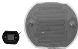
FIGURE 8.1 Light sensor components. (From Wang, J., et al., 40th IEEE/ACM Design Automation Conf. , pp. 66–71, 2003. With permission.)
