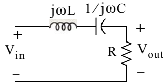
Figure 11.8. Basic band-pass RLC network
