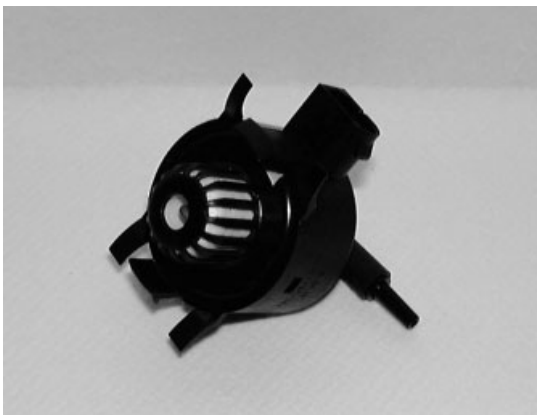
Fig. 7.5.24 Sensor with plastic housing, snap-in design, NTC directly exposed to air, heat radiation shield, additional port for air flow for sensing passenger-compartment air temperature
