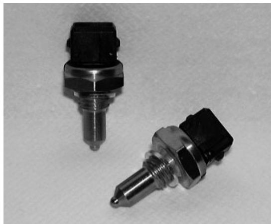
Fig. 7.5.11 Standard sensor with low response time and preassembled aluminum gasket for sensing oil and water temperature up to 170°C in engine and gearbox
