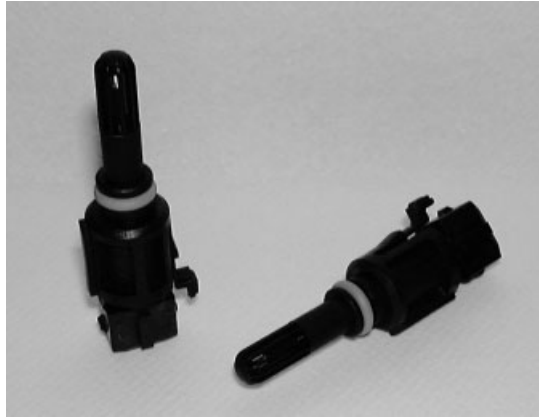
Fig. 7.5.19 Sensor with plastic housing, NTC with direct air contact protected by cage, snap-in design for quick assembly for sensing intake-air temperature in passenger cars
