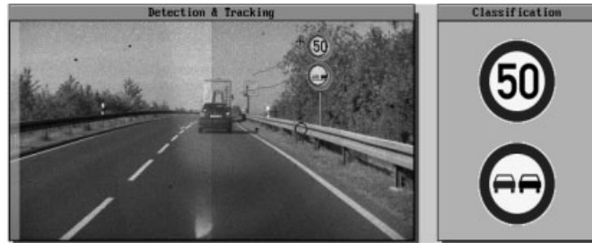
Fig. 7.8.14 Traffic sign recognition: camera image with tracking lines and recognized signs
