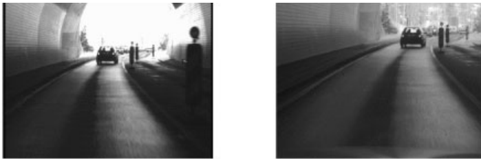
Fig. 7.8.6 Comparison of the dynamic behavior of a charge-coupled device sensor (left) and a nonlinear complementary metal-oxide semiconductor sensor (right)
