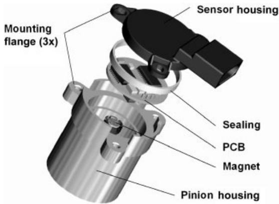
Fig. 7.11.30 Example of a steering-angle sensor using anisotropic magnetoresistance (source: Bosch)
