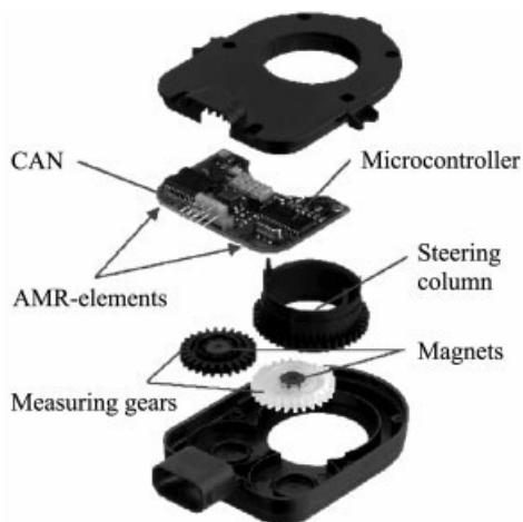
Fig. 7.11.29 Steering-angle sensor using the 180^\circ anisotropic magnetoresistance sensor technology (source: Bosch)
