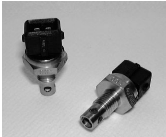
Fig. 7.5.20 Sensor with metal housing, NTC with direct air contact, protected by cage for sensing intake-air temperature in passenger cars
