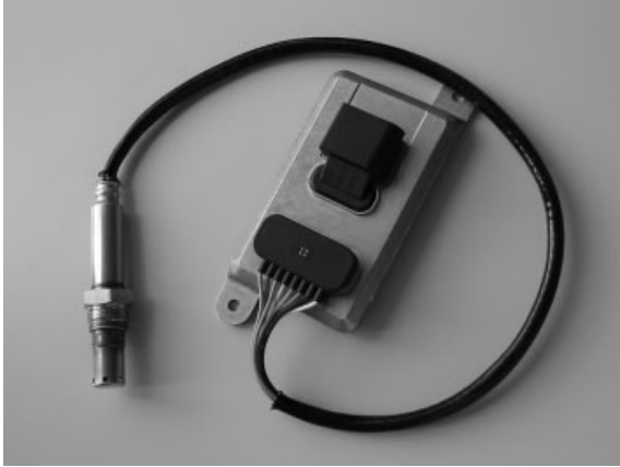
Fig. 7.16.7 The 'smart NO x sensor' made by NGK Insulators (left hand side); electronic control unit made by SiemensVDO Automotive (right hand side)
