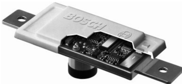
Fig. 7.7.6 24 GHz short-range radar sensor. The high frequency circuit is on the rear side of the substrate. On the right the antenna patches are displayed
