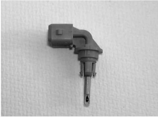
Fig. 7.5.22 Sensor with plastic housing, snap-in design, NTC directly exposed to air for sensing intake-air temperature in passenger cars
