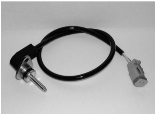
Fig. 7.5.18 Sensor with brass housing on media side, front side O-ring, cable exit, flange assembly for sensing fuel and coolant temperature in commercial vehicles
