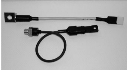
Fig. 7.5.25 Two sensors for measurement of metal temperature: upper sensor for battery temperature measurement, lower sensor for cylinder head temperature in air-cooled engines
