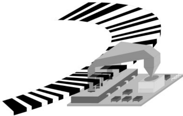
Fig. 7.11.13 Steering-angle sensor principle as a separate optical sensor head (source: Valeo)
