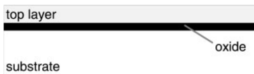
Fig. 5.1.11 Cross section through an SOI wafer
