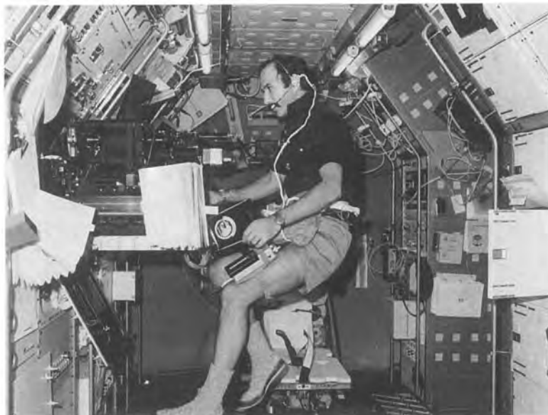
Figure 13-17. The German/European SPACELAB D-1 mission (30 October–6 November 1985), which was under operational management of the German Space Research Institute DLR, was the fourth flight of the ESA-developed SPACELAB with the Space Shuttle. The photograph shows the scientist astronaut Wubbo Ockels (ESA) working with the fluid physics module designed for experimentation with open fluid columns. (Photograph: DLR/ESA).
