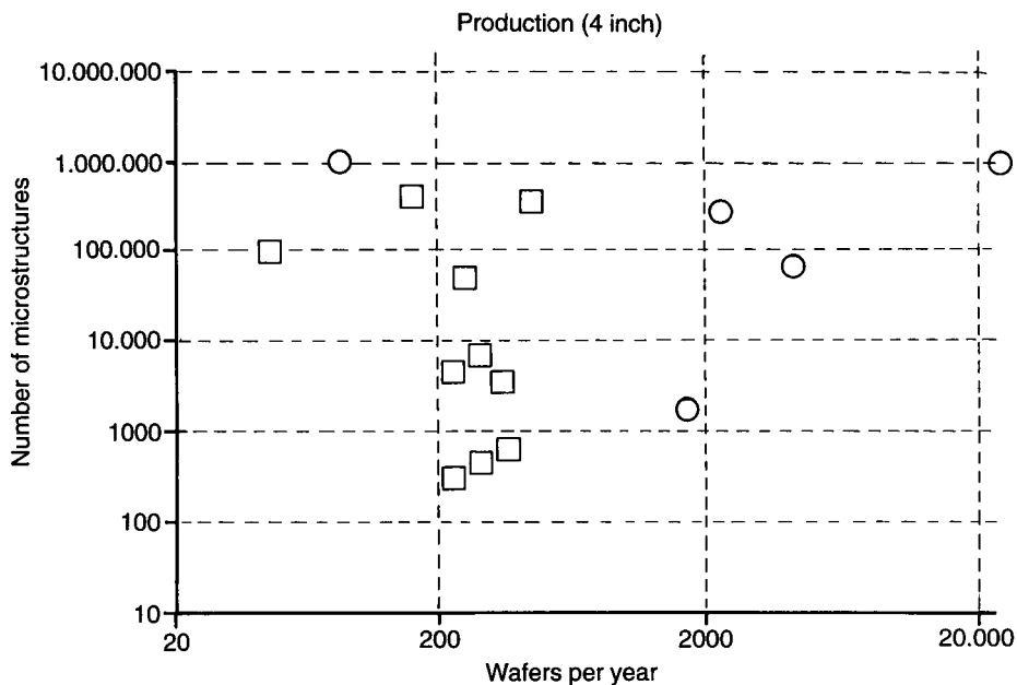
Figure 2-1. Annual number of microstructures and annual number of wafers for various recent industrial demands treated by a 4-inch microsystem service centre.
