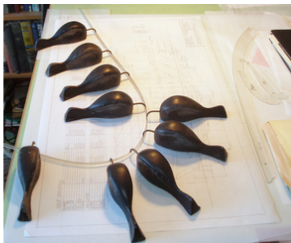
Figure 4-11. Splines were originally created using bendable wood and “ducks” and were used as a draftsman’s tool to fit curves (photo courtesy of Bob Perry)
