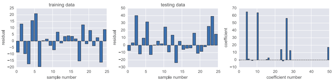
Figure 15-5. The residuals of the LASSO-regularized regression model with cross-validation for the training data (left) and the testing data (middle). The values of the coefficients for the 50 features are also shown (right).
