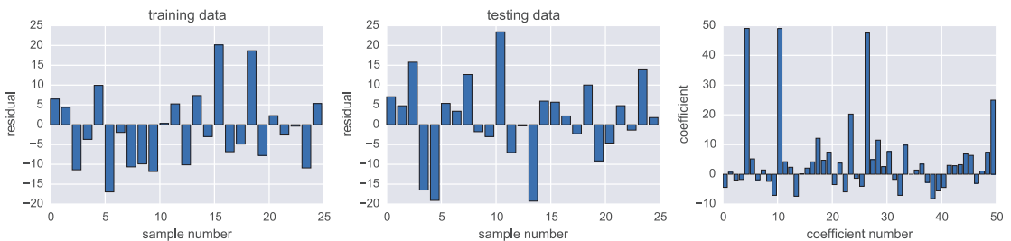
Figure 15-6. The residuals of the elastic-net regularized regression model with cross-validation for the training data (left) and the testing data (middle). The values of the coefficients for the 50 features are also shown (right).
