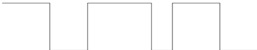
Fig. 1.6 NRZ-L N Nonreturn to zero level representation code
