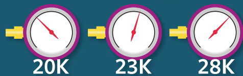
Torqued Nuts and Bolts clamp variation +/- 40%*
