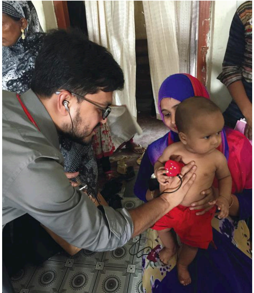
A health worker in Bangladesh listens to sounds from a boy’s lungs with the help of the Johns Hopkins smart stethoscope, which cancels out extraneous noise and identifies telltale signs of pneumonia. (Credit: Dr. Eric D. McCollum)
