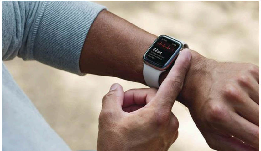
The latest Apple Watch can measure a wearer's electrocardiogram. These types of features can become lifesaving tools as they increase in accuracy.
