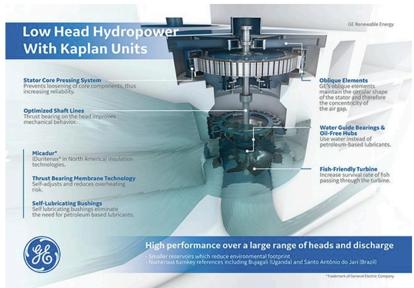
Kaplan turbines are reaction turbines used for low to medium heads of 1.5 to 20 meters, and medium to high flows of 3 m 3 /s to 30 m 3 /s. (Courtesy: GE)
