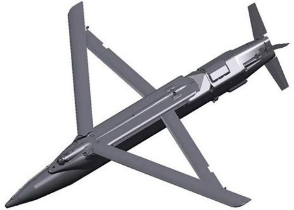
The GBU-39/B Small Diameter Bomb (SDB) from Boeing is a 250-lb precision-guided glide bomb. It was designed to let combat aircraft carry several more bombs than what was one standard. For example, most U.S. Air Force aircraft can carry four SDBs in place of a single 2,000-pounder. The bomb is highly accurate and can guide its descent using inertial navigation or GPS, and home in on targets using radar, infrared, and semi-active laser guidance.
