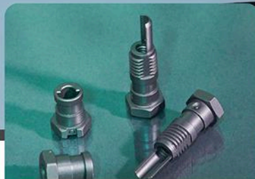
A male fool-proof device and a female polarizer made for an electric connector assembly.
