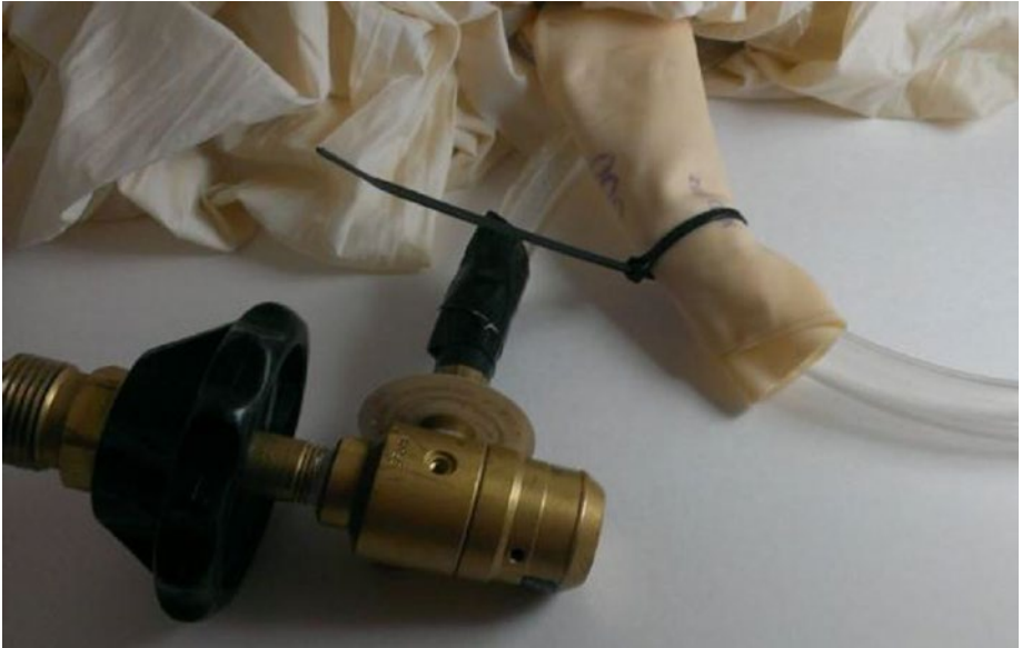
Figure 11-2. Regulator-to-balloon neck setup
