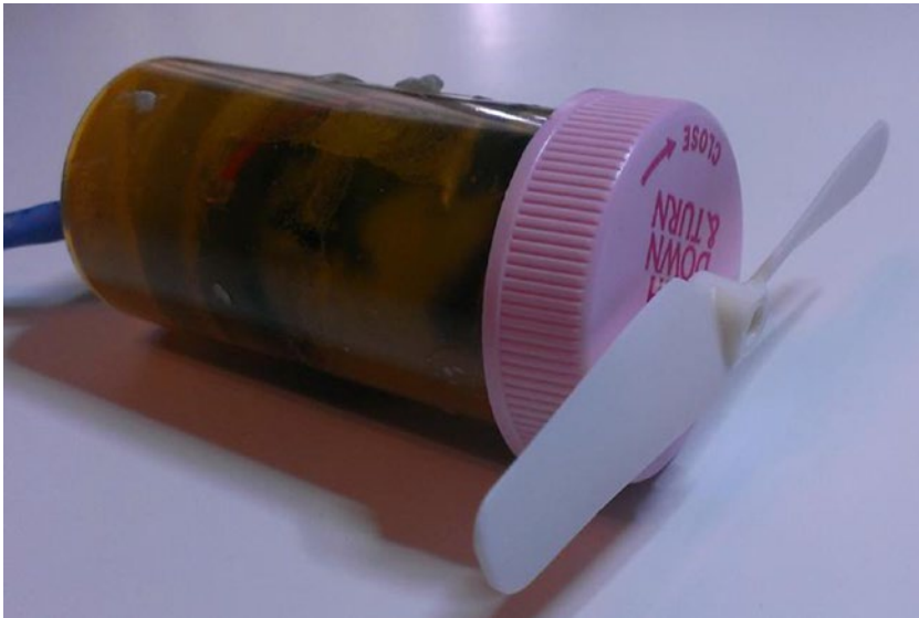
Figure 12-16. Waterproofed motor, ready for mounting
