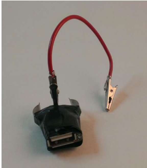
Figure 10-5. Hacked car charger
