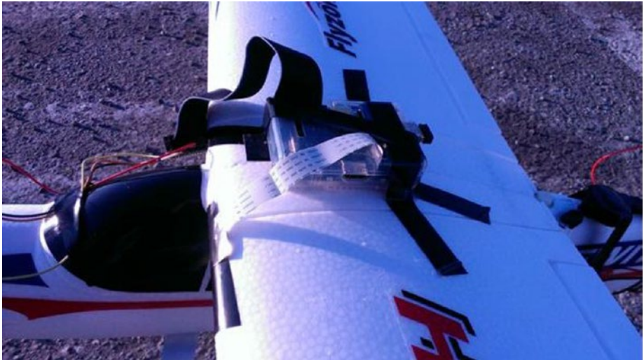
Figure 10-8. Closeup of Pi on plane's wing
