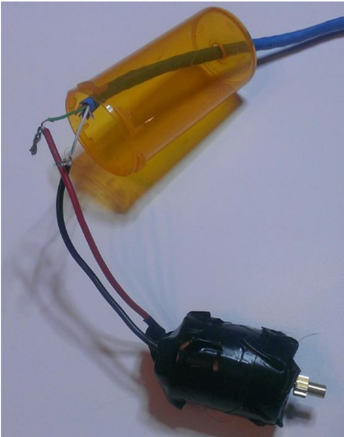
Figure 12-13. Motor ready to be inserted into pill bottle
