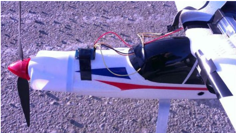
Figure 10-7. Closeup of GPS unit on plane's nose
