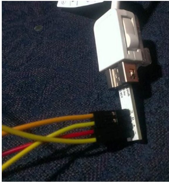
Figure 12-5. Correct positioning of Wiichuk adapter
