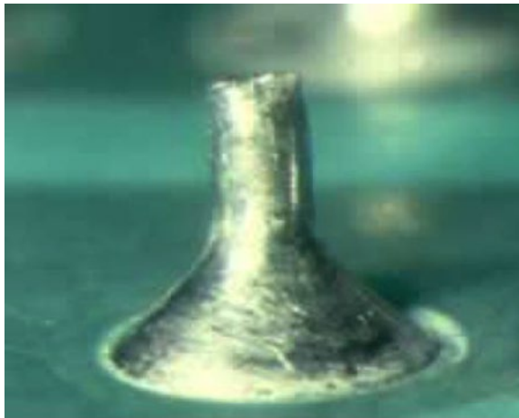
Figure 4-19. Good solder joint
