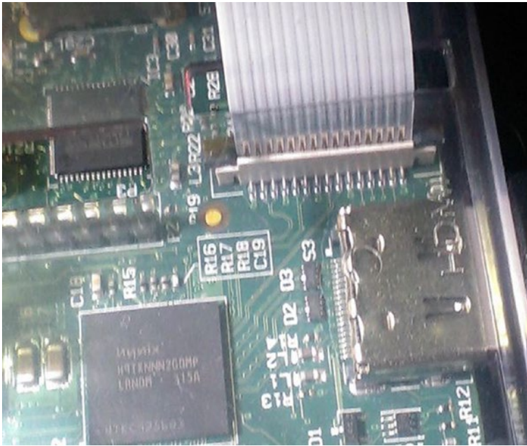
Figure 12-2. Connecting the Pi’s camera cable
