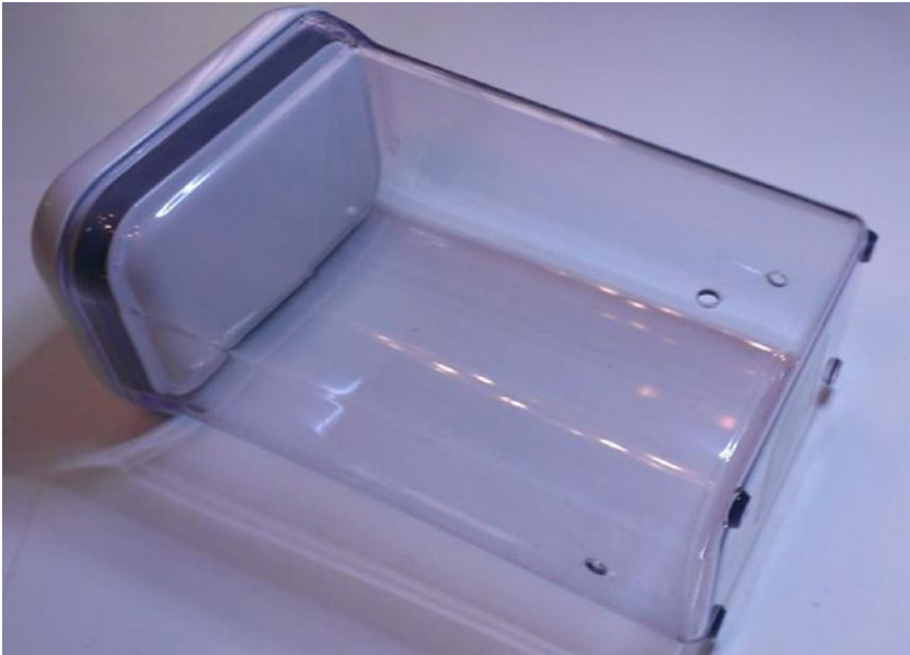
Figure 12-11. Waterproof Pi enclosure
