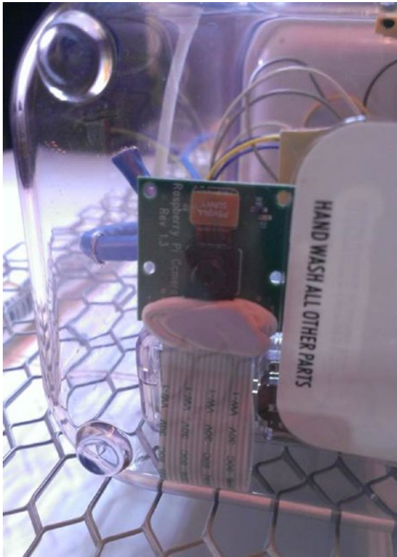
Figure 12-19. Pi camera placement in enclosure
