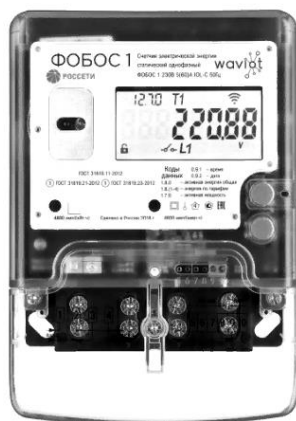
1.6.4-rasm. O‘rnatilgan radio modulli aqlli hisoblagich
