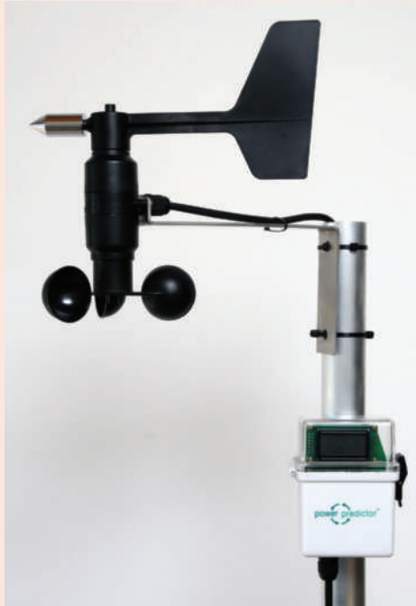
The device is called a 'Power Predictor', it is a combined wind and solar power measuring device that collects local data from the site where it is mounted.
