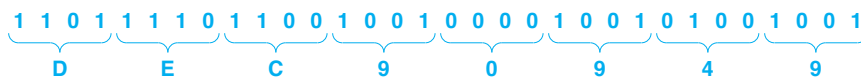
Figure 3.5 Illustration of the relationship between binary and hexadecimal. Each hex digit represents four bits.
