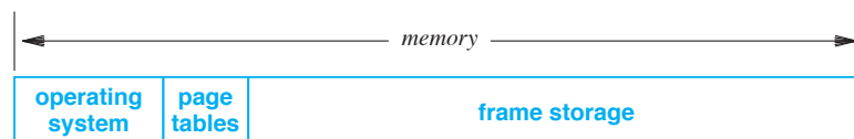
Figure 13.12 Illustration of how physical memory might be divided in an architecture that stores page tables in memory. A large area of physical memory is reserved for frames.
