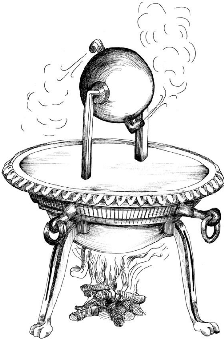
An aelopile – the first steam engine as described by Hero of Alexandria in ad 50
