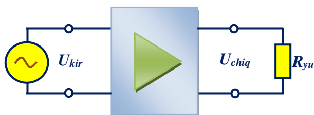
1.4- rasm. Kuchaytirgich ulanishining tuzilish sxemasi
