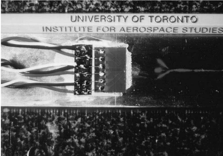
FIGURE 1.6. First fiber optic strain-rosette based on three intrinsic Fabry-Perot interferometric sensors (right side) shown against a conventional resistive foil strain rosette (left side). Both are bonded to a small aluminum beam and placed beside a pen to demonstrate the scale.
