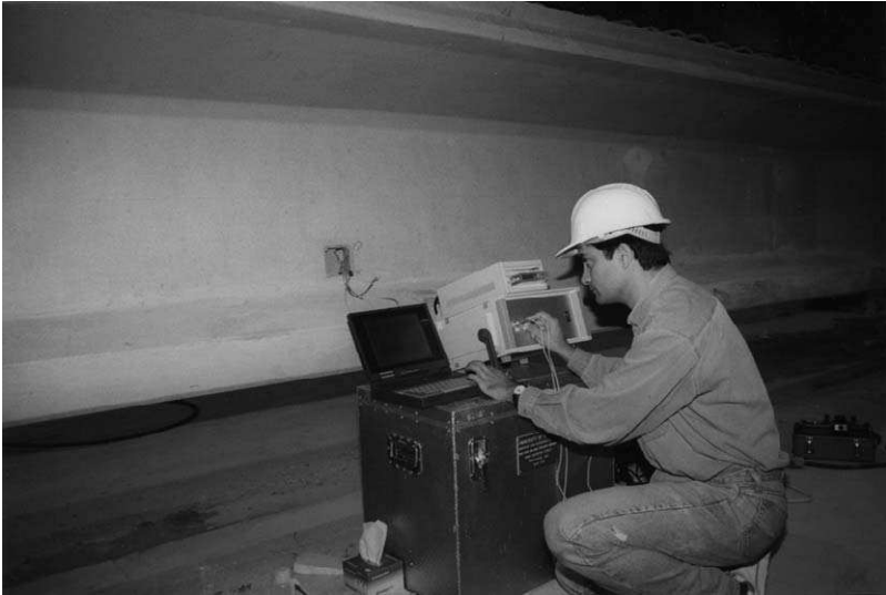
FIGURE 9.40. Testing of the embedded FBG sensor after fabrication of the hot girder for the Beddington Trail Bridge. Used with permission, ElectroPhotonics Solutions Corporation.
