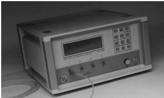
FIGURE 9.4. Photograph of the ElectroPhotonics, four-channel fiber optic grating strain indicator unit, model FLS-3500. Used with permission, ElectroPhotonics Solutions Corporation.
