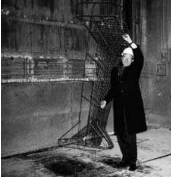
FIGURE 8.11. A section of CFRP shear reinforcement being carried by Professor Urs Meier, demonstrating its light weight in comparison to its steel counterpart. Used with permission, ISIS Canada.
