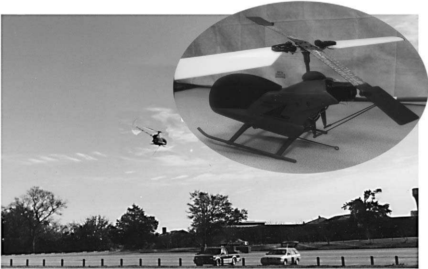
FIGURE 1.3. Small remotely piloted helicopter fitted with piezoelectric adaptive blades that can be made to change the pitch angle of the blade by application of the appropriate voltage. From Barrett, R., Schliesman, M., and Frye, P., "Design, Development and Testing of a Mini Solid State Adaptive Rotorcraft," Proceedings of the 4th Annual Society of Photo-Optical Instrumentation Engineers, SPIE , Annual Symposium on Smart Structures and Materials, San Diego, CA, 3–6 March 1997.
