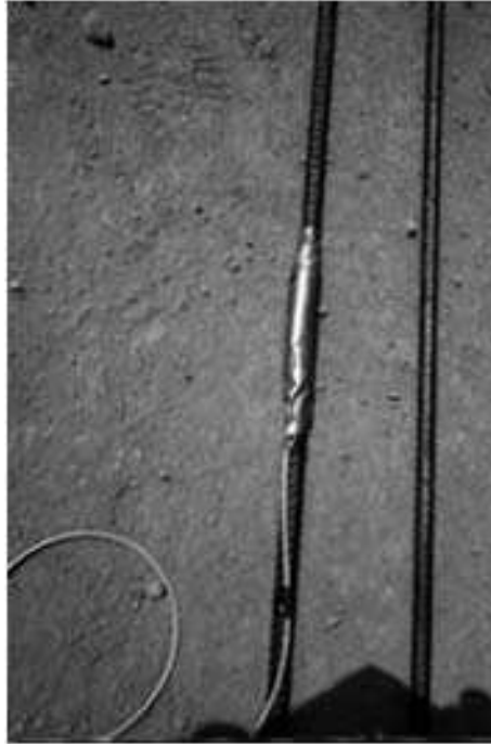
FIGURE 8.7. Steel rebar instrumented with a surface bonded fiber optic sensor and ready for installation within a concrete structure. Clearly seen is the tape covering the protective butyl rubber sheet and the tough optical fiber cable lead to the sensor.
