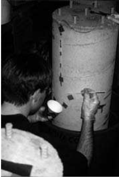
FIGURE 8.5. Surface mounting of a fiber optic Bragg grating sensor on the outside of a concrete column.
