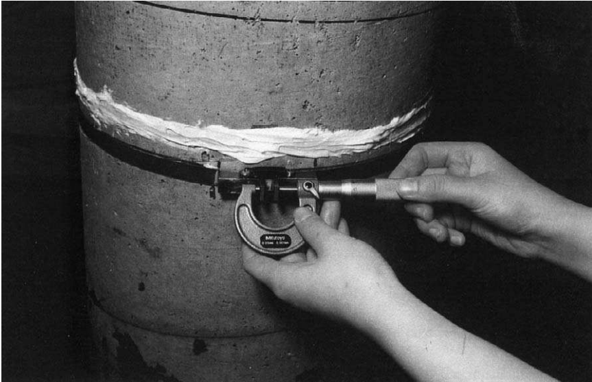
FIGURE 10.43. Close-up view of concrete column instrument with a long gauge-length fiber optic strain sensor (protected by white silicon caulking) and a conventional mechanical expansion collar. From MASC Thesis, C. Lee, 1998, Civil Engineering, University of Toronto, Canada.
