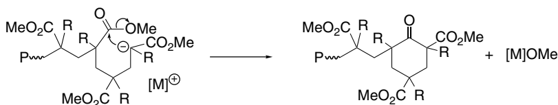
SCHEME 23.3 Intramolecular cyclization for PMA (R = H) and PMMA (R = Me) (P = polymer chain and M = metal cation).
