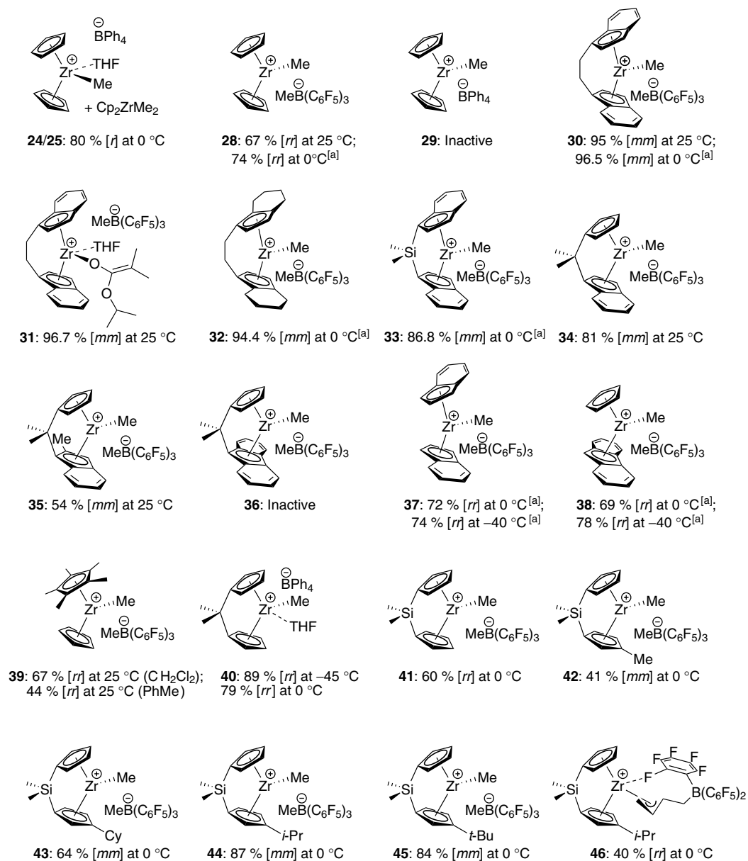
FIGURE 23.9 Cationic zirconocene initiators for MMA polymerization and the resultant PMMA microstructures ([a] = in the presence of ZnEt 2 ).
