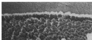
Fig. 4.2. Top edge of cross section of polyamide-hydrazide asymmetric gel membrane taken by SEM. Reprinted from Polymeric Gas Separation Membranes by R.E. Kesting and A.K. Fritzsche, p 248. Copyright 1993, with kind permission from Wiley
