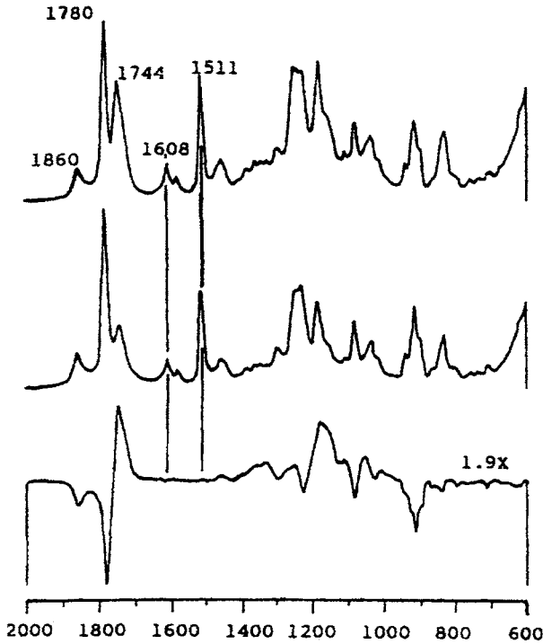
Fig. 4.2. Generation of difference spectrum to characterize crosslinking at 80°C of a stoichiometric mixture of NMA-EPON 828. The samples were crosslinked for 83 min (top spectrum) and 37 min (middle spectrum). The bottom spectrum is the difference spectrum (top - middle).
