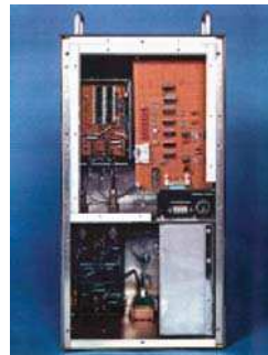
Cosmic Radiation Effects & Activation Monitor (CREAM): "Concorde" version flown on BA Concorde, SAS Boeing 767 and NASA WB-57F (Dyer et al., 1999)
