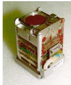
Dose Telescope (DOSTEL, Si dose and spectrometer) measurements onboard space shuttle, space station and onboard aircraft (Beaujean et al., 2005)
