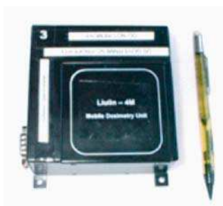
Liulin Si dose and spectrometer measurements onboard space shuttle, space station and onboard several aircraft (Spurný and Dachev, 2002)
