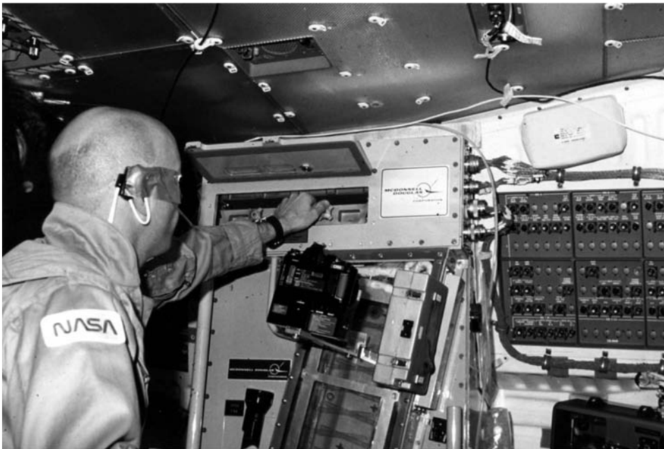
Story Musgrave operates the Continuous Flow Electrophoresis System on Challenger’s middeck.
