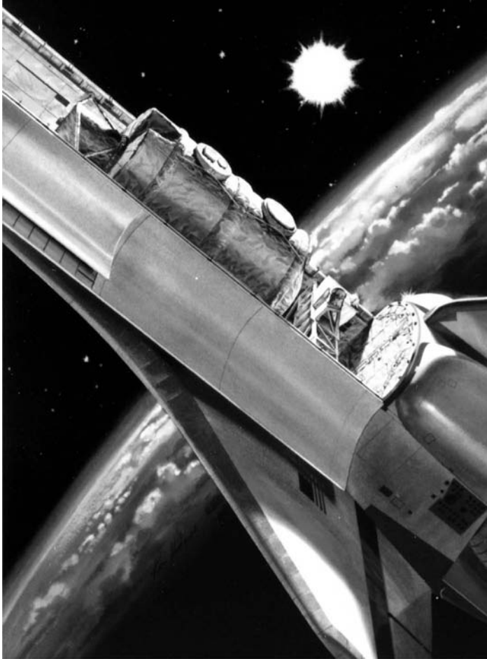
Diagram of the gravity gradient attitude adopted by Challenger during the bulk of STS-51B orbital operations. The Spacelab-3 facility, consisting of the long module and MPRESS, are clearly visible in her payload bay.
