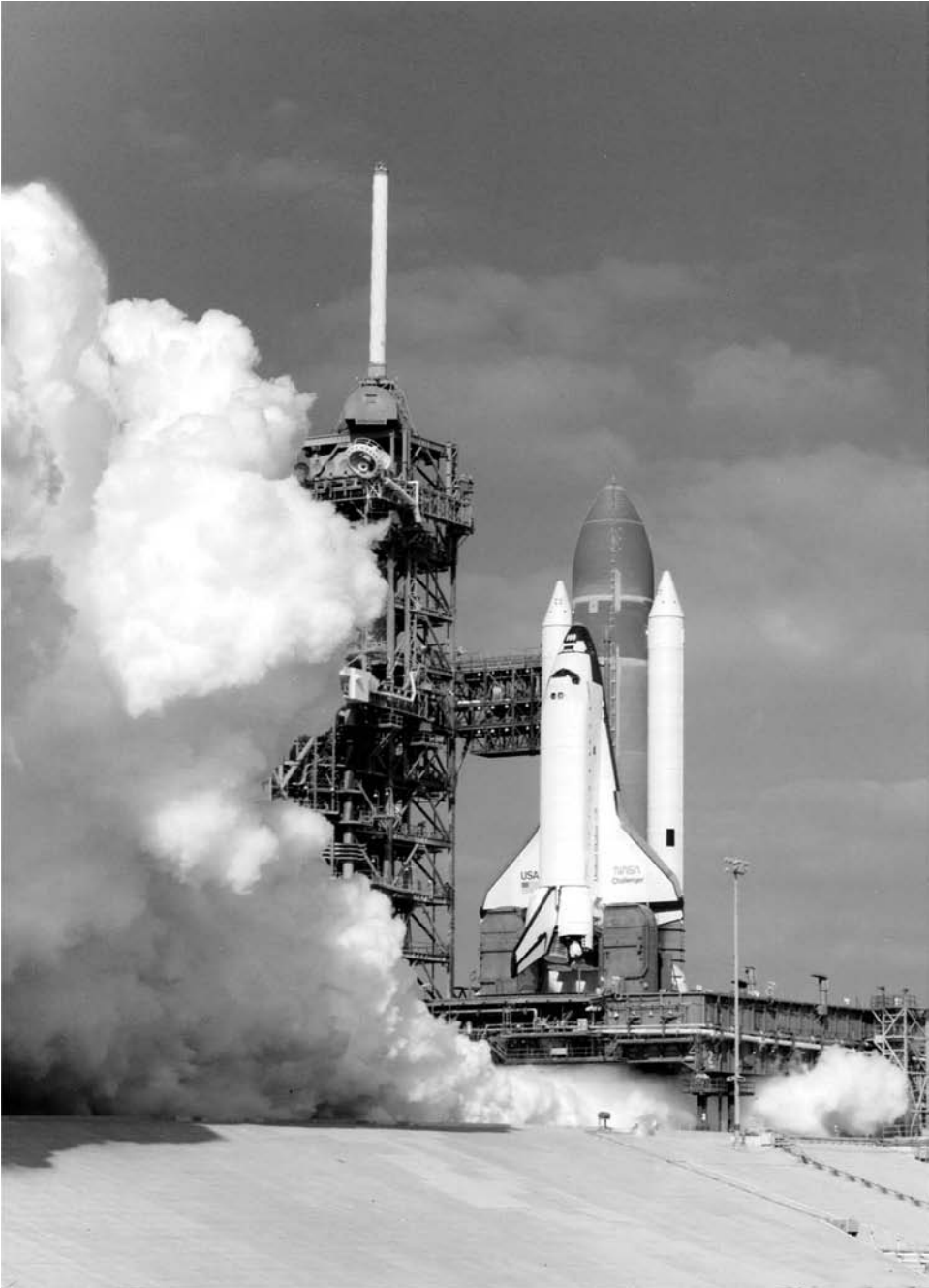
Challenger undergoes the first Flight Readiness Firing of her three main engines on December 18th 1982. Note the unusual 'butterfly and bullet' combination of the Shuttle stack, consisting of the orbiter, External Tank and twin Solid Rocket Boosters.
