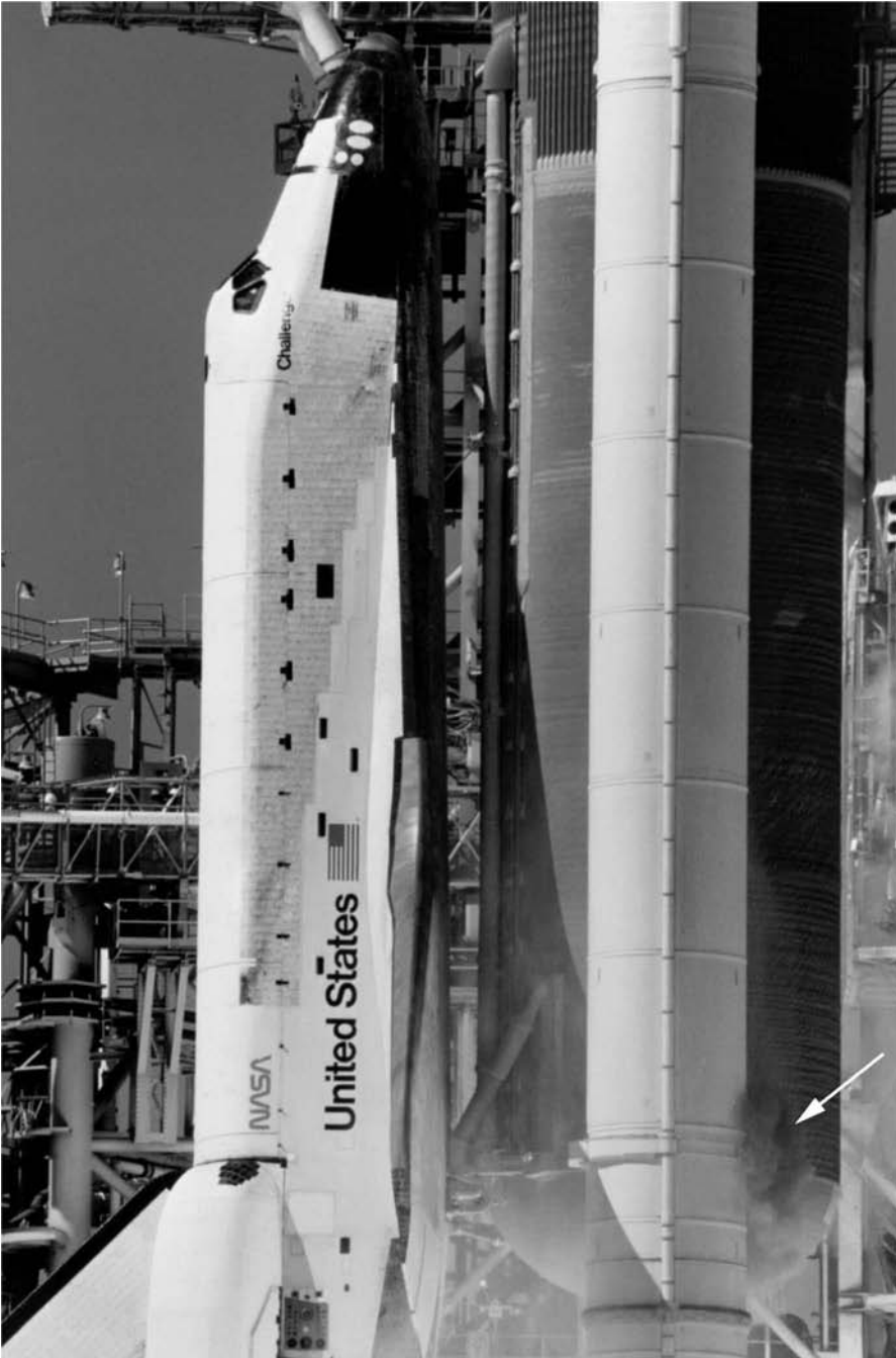
First evidence of a puff of smoke from the right-hand Solid Rocket Booster, milliseconds after STS-51L's lift-off.
