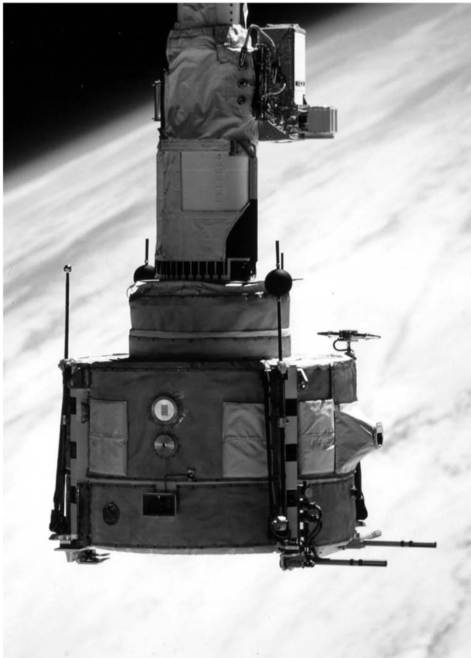
The drum-like Plasma Diagnostics Package (PDP) in the grip of Challenger's mechanical arm during a series of experiments on August 1st 1985.
