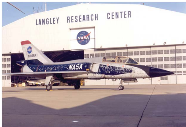
Fig. 2 NASA F-104 Lightning research aircraft. The paint has been burned off in hundreds of locations where lightning strikes hit the airframe
