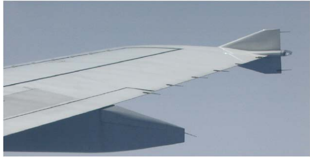
Fig. 3 Trailing edge of a commercial airliner—note the narrow discharge wicks to allow accumulated electrical charges to dissipate. (Photo: R Lorenz)
