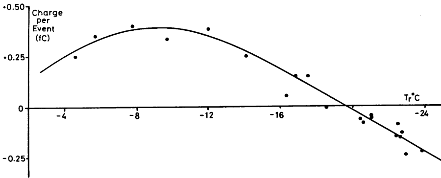
Fig. 5 The charge transferred to a riming graupel pellet by a separating ice crystal following a collision, at constant cloud water content. (Jayaratne 1981)
