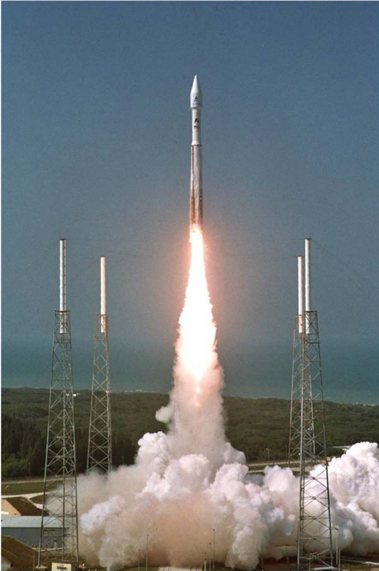
Fig. 5 Atlas-V launch from Kennedy Space Center in Florida. Note the 4 towers to attract lightning away from the launch vehicle itself on the launch pad. Note also the long, luminous (and partly conductive) exhaust which augments any preexisting electric fields. (Photo: NASA)
