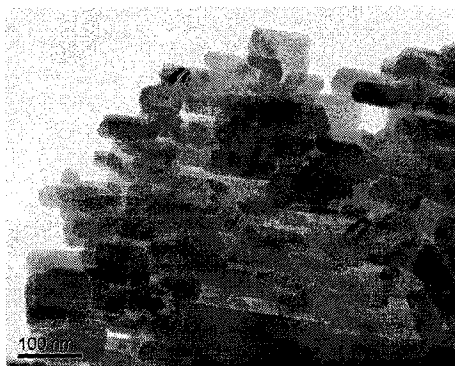
Figure 2. TEM images of the \text{LiFePO}_4 nanorods.
