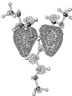
Fig. 4.2.13. Lowest energy unoccupied molecular orbital (LUMO) of the PEG-borate ester.
