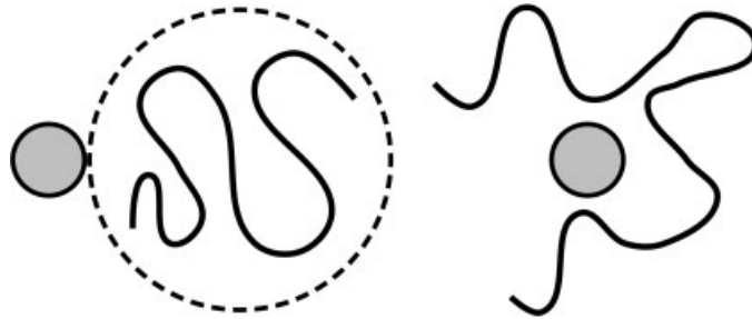
Fig. 2.3 Small colloidal particle interacting with a rigid polymer (left) and with a flexible polymer (right).
