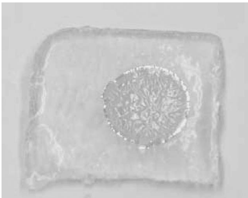
FIGURE 11.11 P Si microcavity sensor after contact-adhesion to NuGel hydrogel.
