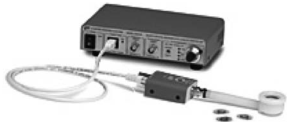
FIGURE 21.4 QCM100. Quartz crystal microbalance analyzer. (From http://www.thinksrs.com/ . Accessed December 20, 2004.)
