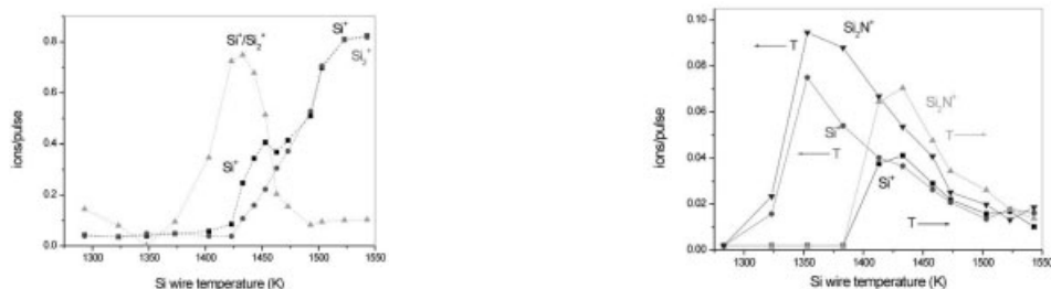
Figure 3.9. Yield and ratio of masses 28( \text{Si}^+ ) and 56( \text{Si}_2^+ ) obtained by ArF laser ionization (left) and of masses 28( \text{Si}^+ ) and 70( \text{Si}_2\text{N}^+ ) obtained by KrF laser ionization (right) as a function of the Si wire temperature. [5, 6]
