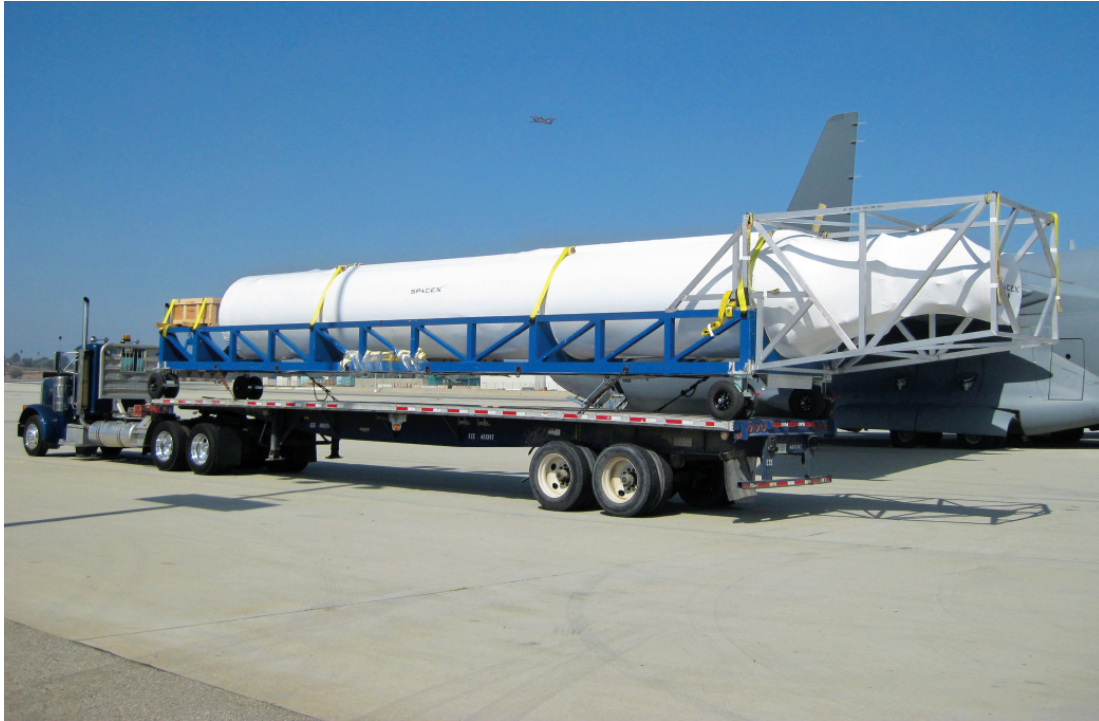
Short on time, SpaceX couldn't wait the month it would take to ship the Falcon 1 to Omelek by barge for Flight Four. Transporting a rocket by airplane is no easy task; here, the Falcon 1 first stage is wrapped for its flight on a C-17 aircraft. (Zach Dunn)
