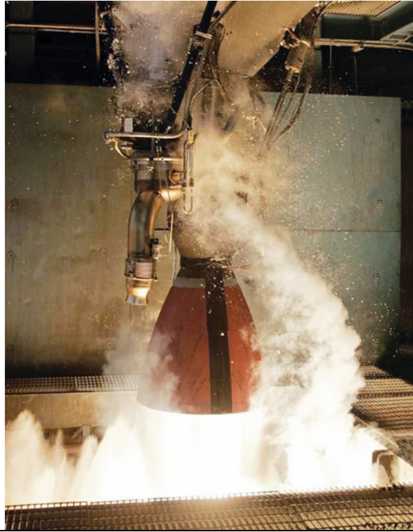
A Merlin rocket engine is test fired in McGregor, Texas. (Tim Buzza)
