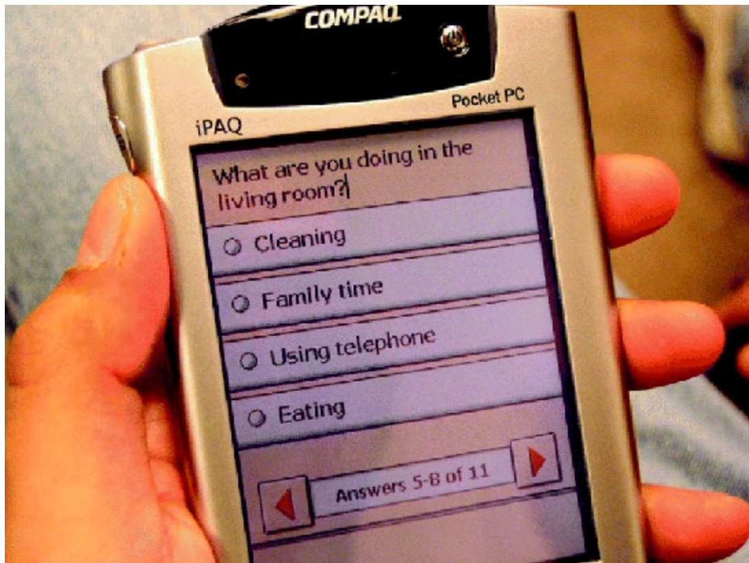
Figure 14.7 An example of a context-aware experience sampling tool running on a mobile device
