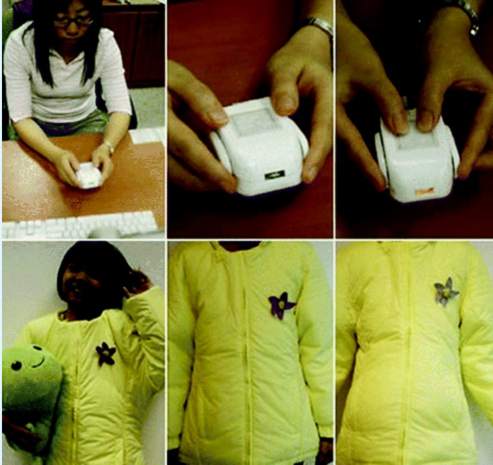
Figure 4.12 Huggy Pajama with mother squeezing the remote device and child being correspondingly squeezed
