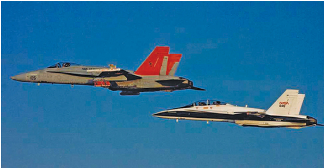
Flying a U.S. Navy F/A-18 with a hydrogen-burning research engine on the wingtip, being chased by a NASA Dryden 2-seater, at Pax River, 1991. (Credit: Chris Hadfield)
