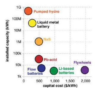
This figure shows the various energy storage methods plotted on an Installed Capacity versus Capital Cost graph. According to Professor Sadoway, the key metrics required for grid-scale storage are (i) cost (<\$150/kWh); life span (>10 years); and energy efficiency (>80 %)—all of which are achievable by liquid metal batteries.
