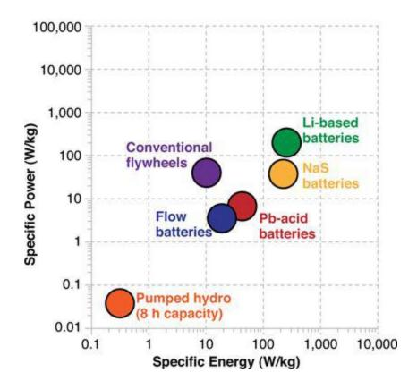
The graph shows the relative specific power (amount of current the battery can deliver) versus specific energy (energy per unit mass).
