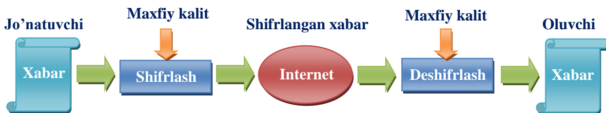
4.9- rasm. Simmetrik shifrlashga misol
